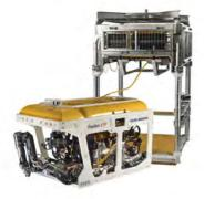
The Seaeye stainless steel TMS type 8 uses a bail arm to spool up to 200m of tether on and off a drum controlled by the ROV pilot. The TMS height can be adjusted to accommodate different tool skids.
