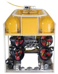
PANTHER-XT PLUS SHOWING TOOL SLEDGE COMPARTMENT
